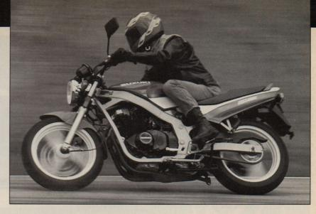
than two valves per cylinder, it doesn't have gear-driven cams, hydraulic lifters, or anything else that a 1966 Honda CB450 didn't have. And yet the power is very satisfying. Low-end torque hits with a healthy surge at about 4000 rpm, and even if the bike is through making power well before its 11,000-rpm redline, a six-speed gearbox lets you continue
