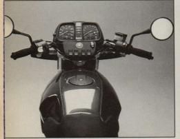
The K75's instruments and warning lights are neat and easily readable. Those rockers below the ignition switch are dummies that can be replaced with real switches when accessories are added.
