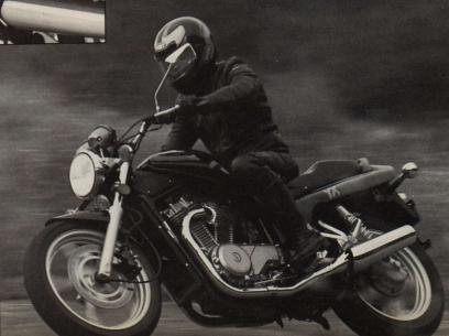
crankpin offset from 45 to 75 degrees in hope of creating a smoother-running motor. But just as production began, American Suzuki engineers decided that the new offset resulted in less mid-range power, as well as a too-sanitized exhaust note, one that didn't sound very V-Twin-like. Presto, now the U.S. models come with the 45-degree offset, while the rest of the world gets the 75-degree staggered crankpins.
