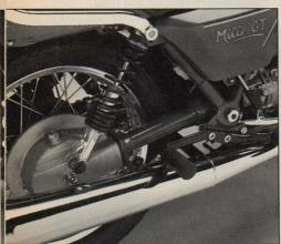
The Moto Guzzi retains that firm's characteristic shaft drive. Though not up to flogs at sportbike speeds, its Koni shocks are more than adequate for back-country cruises.
