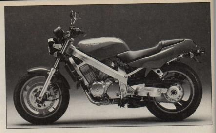
Riding the Hawk further demonstrates that it is, indeed, something more than an ordinary standard motorcycle: The footpegs are mounted high and to the rear, more like a sportbike than a standard, and its handling is sharp, accurate, quick and responsive. Its suspension—a single shock rear and conventional fork—provides excellent control until near-racetrack speeds are reached, and it does an above-average job of isolating the rider from bumps.
