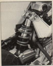
Suspension loads from the Hawk's beefy single-sided swingarm— known as a Pro-Arm, in Hondaspeak—are fed into the bike's deCarbon-type single shock.
