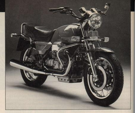
twin, 30mm Dell' Orto carburetors, though our Italian connections tell us the cure for that is simple and cheap. And, as you rev the engine, the torque reaction from its beefy crankshaft and 12-pound flywheel rocks the bike to the right, but this is more an oddity to be noticed at stoplights than a problem that causes handling glitches, at least at the speeds the Mille likes best.
