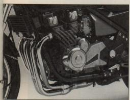
The Zephyr's 550cc engine, a nottoo-distant relative of the old KZ550 motor, is air-cooled and has but two valves per cylinder.
