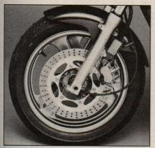
Lockhart fork springs and a Metzeler Comp K Laser tire offer a taut ride and more front-end feedback. The stock disc and dual-piston caliper perform admirably.
