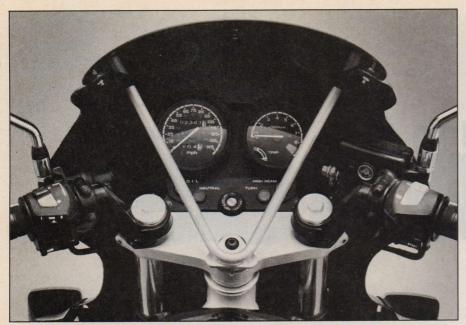
The Targa fairing channels air directly at the rider's head and shoulders, though it's not turbulent enough to cause major noise or comfort problems.
