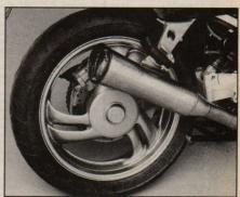
Though louder, the stainless steel Super-Trapp exhaust provides more midrange punch than the stocker and is lighter. Metzeler ME1 rear tire sticks tenaciously.
