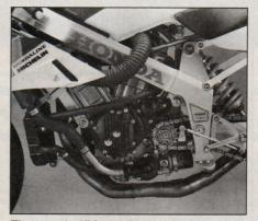
The massive RS750 dirttrack ignition eliminates the Hawk's battery and allows the engine to rev to 12,000 rpm. The stock footpegs are replaced with RS250 items.
