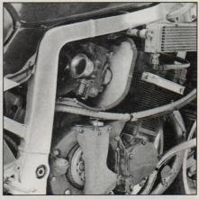
Yosh's Superbike motor puts out 137 horsepower with a 5000-rpm-wide powerband. The racing dry clutch is similar to the '86 GSXR750 LTD's unit but lighter.
