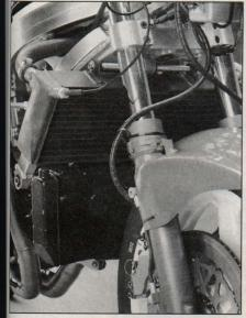
Perhaps Velasco's best work, the dual radiators and revised cooling system contain the heat produced by the 700cc Hawk, dropping coolant temp over 70 degrees.
